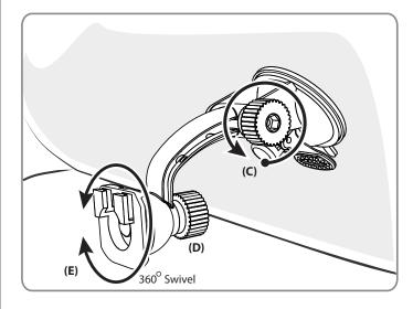
2. Attach the cradle (F) to the pedestal head (E) by sliding the Dual T-tabs on the head of the pedestal into the dual T-slots on the back of the cradle.
