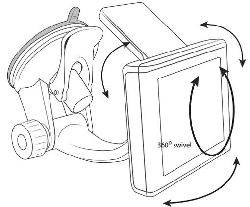
6. To remove, hold the pedestal with one hand and firmly pull Nuvi away from pedestal with your free hand.
